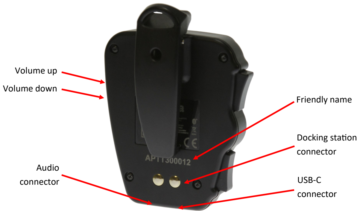
Figure 2: Rear view and connectors
